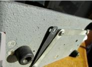
ing metal strips joined together. Insulation is necessary to prevent these bare conductors from shorting to the base, but insulating them from each other was cause for the open circuit on the dah side. The fix was to correct the assemblers' mistake, which makes me think that this bug has patiently waited about 54 years to operate.
