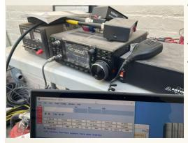
The Yale I-EEE student branch is the main face of current student ham radio at the university. They operate a small station on the northern half of the Yale University Campus. We currently have VHF/UHF capability with an ICOM IC-7300 and a pair of 2MCP14 + 436CP30 M2 Antennas.
