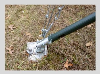
(1) First gen. tripod mast swivel leg mount used with 41 ft tripod
