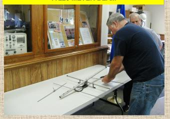
The 6 Meter .3 element was beam installed at the Firehouse Saturday. Very flat across the band, less than 2.0 SWR without tuning 50.1 to 54.0 MHz.
