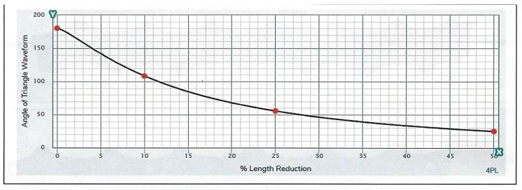
Figure 1. Plot of various data points representing antenna-wire length reduction vs. angle of waveform. (Graphic output produced by MyCurveFit.com)
