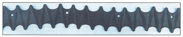
Photo C. An example of Sabertooth wire made with 25-degree wire angles. This version provides 50% end-to-end antenna-wire shortening.
