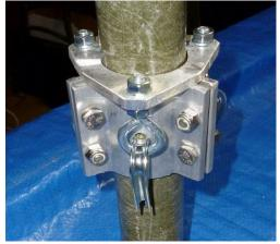
Mast joint clamp with aluminum guy ring
