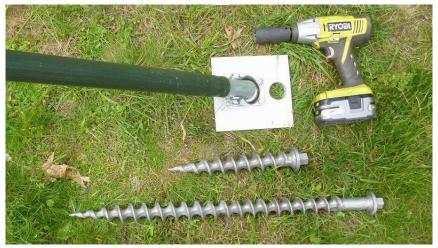
A 1/2 Inch electric impact wrench drives the anchors easily
