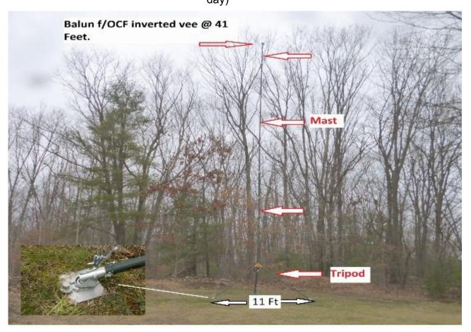
I'm a big fan of those Army surplus masts (fiberglass and aluminum) that were made for tent poles and other structures used by the armed forces. Coupled with one of the available tripod mounts, they are excellent for use as portable or temporary antenna masts.
