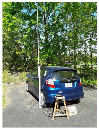
We're using WB1GYZ's 5/4 wave antenna for the fox transmitter. The top of the antenna is fourteen feet off the ground. Though our coverage in Wallingford has been pretty good, this can only help.
