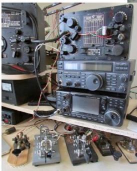
ing metal strips joined together. Insulation is necessary to prevent these bare conductors from shorting to the base, but insulating them from each other was cause for the open circuit on the dah side. The fix was to correct the assembler's mistake, which makes me think that this bug has patiently waited about 54 years to operate.
