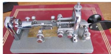
I wondered if the synthetic clock oil applied to the pivot/bushing points created electrical resistance. That was a long-shot guess but I was running out of possibilities. It was time to stop guessing and get an ohm meter to trace the circuit.
